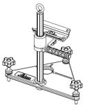
The Trivet Assembly (746158) includes the mounting bracket that is attached to the bottom of the laser.
